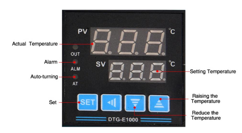
Operation: Press the set key "SET"; The above line display SU; The bottom line display the set value; Then press the shift key or plus, minus key to set temperature. If set at 100 °C, please press the set key to return to the using of self-tuning after the bottom line display 100.
